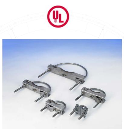
APPLICATION: Cast U-BOLT bonding clamp provide 1-1/2" of surface contact on pipe and cable. Use with all full size conductors. Fits pipe sizes  $\frac{1}{2}$ " to 6-3/4".
