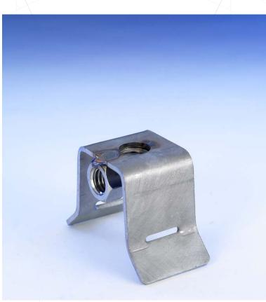
APPLICATION: This saddle base is used for securing an air terminal to pipes large in diameter. Saddle Base, Stainless Steel w/ 1/2" Nut & Hose Clamp (Fits up to 10" Pipe) Mounts Vertical & Horizontal. Please specify the pipe size when ordering, and additional hose clamp may be needed for pipes larger than 10" DIA.
